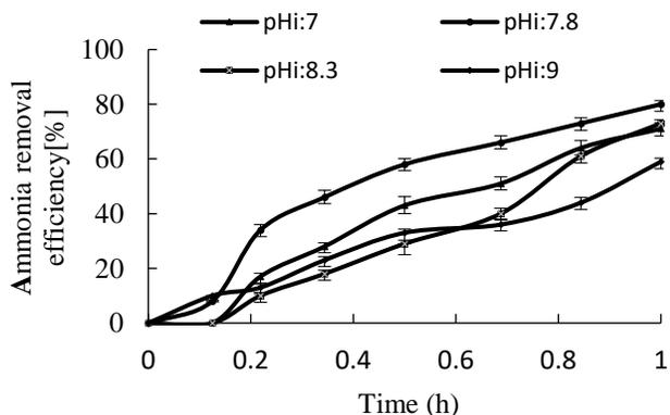
**Figure 5.** Effect of pH on ammonia removal using wastewater from depot 93 of the Shiraz Petrochemical plant.
