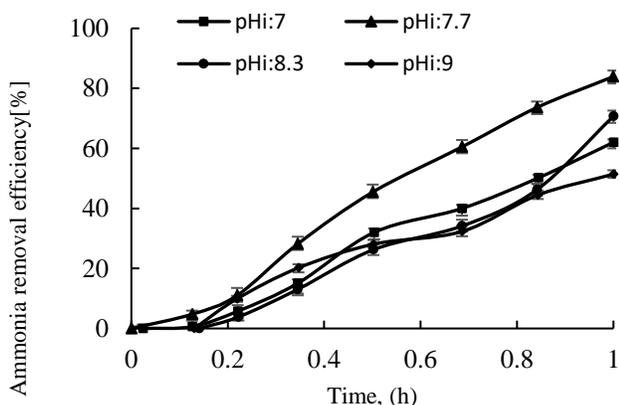
**Figure 4.** Effect of pH on ammonia removal using Watson medium.
