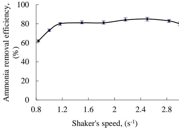
**Figure 6.** Effect of shaker speed on ammonia reduction of the wastewater of depot 93 of Shiraz Petrochemical plant.
