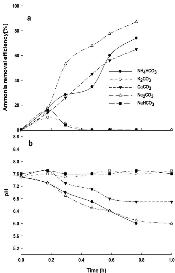
**Figure 2.** Effect of various carbon sources on nitrification of wastewater of depot 93 of the Shiraz Petrochemical plant.
