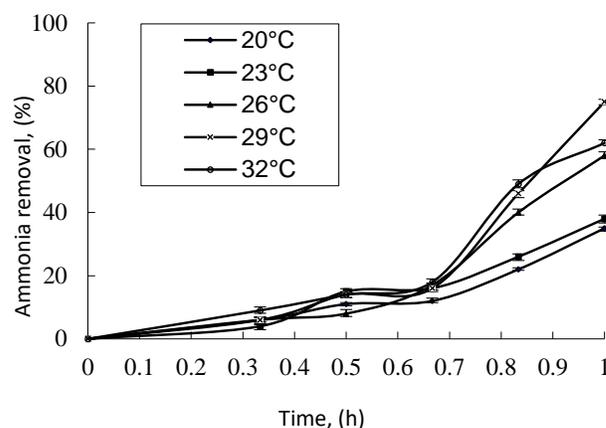
**Figure 3.** Effect of temperature on the ammonia removal using the wastewater of depot 93 of the Shiraz Petrochemical plant.
