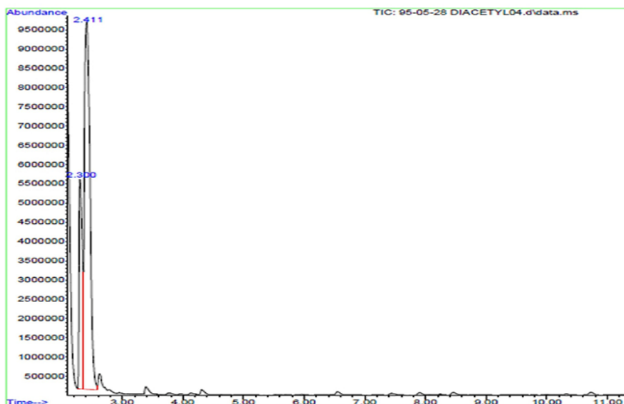
Figure 4: Results from Gas Chromatography Confirmed the Successful Extraction of Diacetyl
