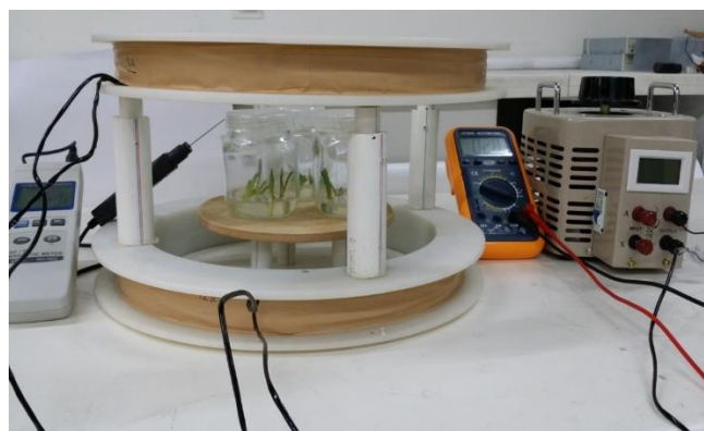
Figure 1: System for Applying an Alternating Magnetic Field to a Plant
